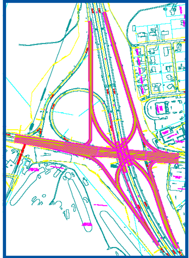
Drawing of Single Point Urban Interchange alternate for the Plank Road Interchange. (For additional drawings and mapping please visit the project website at www.plankroadinterchange.com .)
